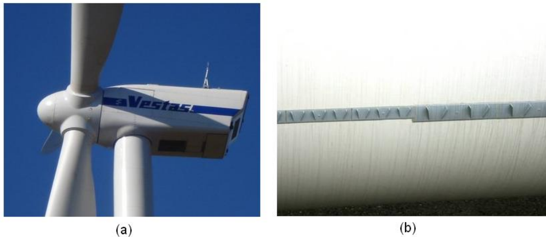
Fig. 1: Wind turbines utilizing (a) pitch control (World News, 2010) (b) vortex generators (Wapedia, 2010)
