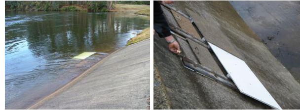
Fig.5 Test plate installation in canal
